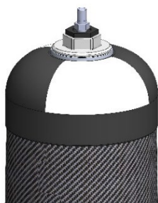
Figure 4: Cylinder with bicycle-type valve and internal pressure
